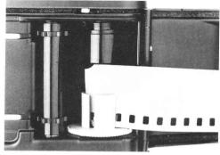
Pick up the film cartridge as illustrated above. The emulsion side points to the viewer. Push the end of the film obliquely from above into one of the slots of the take-up spool. Ensure that the end of the film is fully gripped by at least one lug and protrudes under the next lug.
