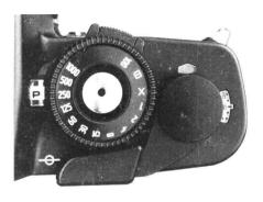
automatic program with LEITZ largefield integrating measurement. Set the minimum aperture of the lens.
