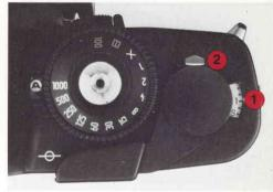
Close the camera by snapping the camera back shut. Release the shutter. Transport the film through one frame and again release the shutter. Transport the film once again. The camera is now ready for operation. The film counter (1) points at 1. It counts forward to "36". For the various lengths of film the numbers "20", "24", and "36" are marked in red.
