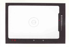
Measurement with the working aperture The 35 mm PA-CURTAGON-R f/2.8, the long-focal-length lenses from 400 mm, the focusing bellows-R, the extender-R 2x for the LEICAFLEX SL/SL 2 and the 3-part ring combination have no automatic diaphragm or no coupling for it. Here the exposure must be measured through the lens aperture used, i.e. through the working aperture. Here the lens aperture is adjusted to regulate the amount of light reaching the measuring cell of the LEICA R4.
