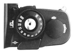
automatic shutter-speed control with LEITZ selective measurement Preselected the desired lens aperture
