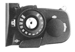
At "X", "B" and "100" the exposure is not measured even when the button cells are inserted. This is indicated in the viewfinder by the lighting up of the upper triangular LED.
